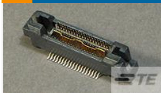
TE Part # 5767119-1 MICT,PLG,038,ASY,.025,TAPE PKG
